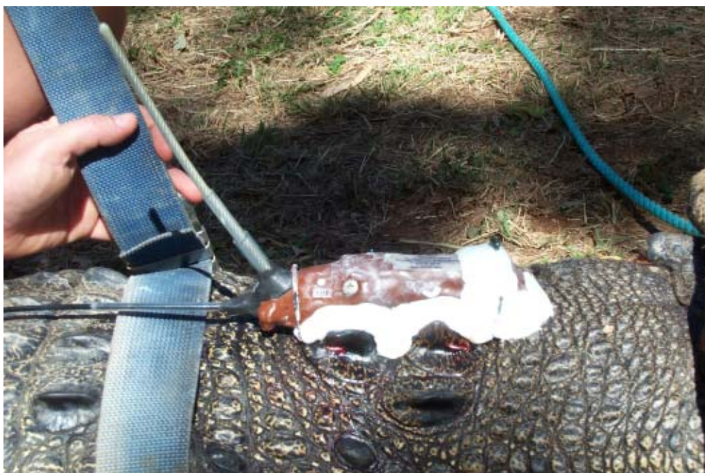
Figure 6. The satellite transmitter attached to "Harriett", showing the epoxy glue and wire bonding the unit to the nuchal shield.
